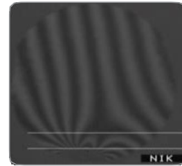
1,000 μm diameter fiber Interference microscope image 1 stripe = 0.01°
